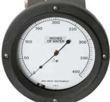
Dry Gauge Design with No Internal Liquid Fill
