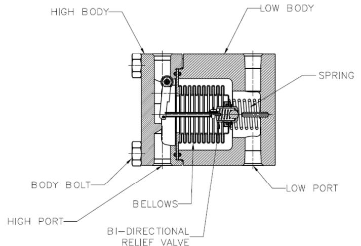
The body halves provide the pressure containment function. They also clamp the sensing element and over-pressure assembly between the body halves, isolating the high side and low side pressures of the system. The high side body half also provides a mount for the torque tube assembly.
