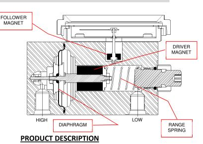
The Model 114 is a differential pressure instrument available as a switch, gauge, or both. A flexible elastomer diaphragm and calibrated range spring are moved by differential pressure. A magnet, coupled with the diaphragm, transmits motion through the wall of the pressure housing to a follower magnet attached to an indicating pointer. The rotation of the follower magnet causes the pointer to track movement of internal driver magnet and indicate differential on the dial scale.
