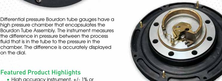
Bourdon Tube Assembly. The instrument measures the difference in pressure between the process fluid that is in the tube to the pressure in the chamber. The difference is accurately displayed on the dial.
